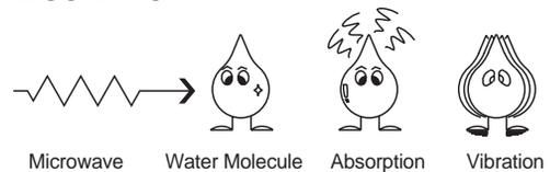
The microwaves cause the water molecules to vibrate which causes **FRICTION**, i.e. **HEAT**. This heat then cooks the food. Microwaves are also attracted to fat and sugar particles, and foods high in these will cook more quickly. Microwaves can only penetrate to a depth of 1½ - 2 inches (4-5cm) and as heat spreads through the food by conduction, just as in a traditional oven, the food cooks from the outside inwards.
