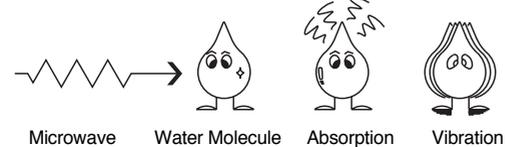
The microwaves cause the water molecules to vibrate which causes **FRICTION**, i.e. **HEAT**. This heat then cooks the food. Microwaves are also attracted to fat and sugar particles, and foods high in these will cook more quickly. Microwaves can only penetrate to a depth of 1½ - 2 inches(4-5cm) and as heat spreads through the food by conduction, just as in a traditional oven, the food cooks from the outside inwards.
