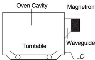
In a microwave oven, electricity is converted into microwave by the **MAGNETRON**.
