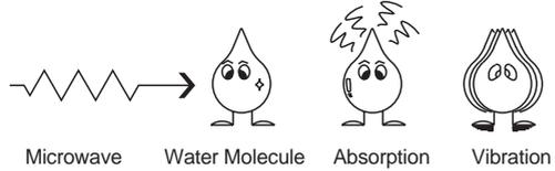
The microwaves cause the water molecules to vibrate which causes **FRICTION**, i.e. **HEAT**. This heat then cooks the food. Microwaves are also attracted to fat and sugar particles, and foods high in these will cook more quickly. Microwaves can only penetrate to a depth of 1<sup>1</sup>/<sub>2</sub> - 2 inches(4-5cm) and as heat spreads through the food by conduction, just as in a traditional oven, the food cooks from the outside inwards.
