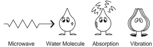
The microwaves cause the water molecules to vibrate which causes **FRICTION**, i.e. **HEAT**. This heat then cooks the food. Microwaves are also attracted to fat and sugar particles, and foods high in these will cook more quickly. Microwaves can only penetrate to a depth of 1½ - 2 inches(4-5cm) and as heat spreads through the food by conduction, just as in a traditional oven, the food cooks from the outside inwards.
